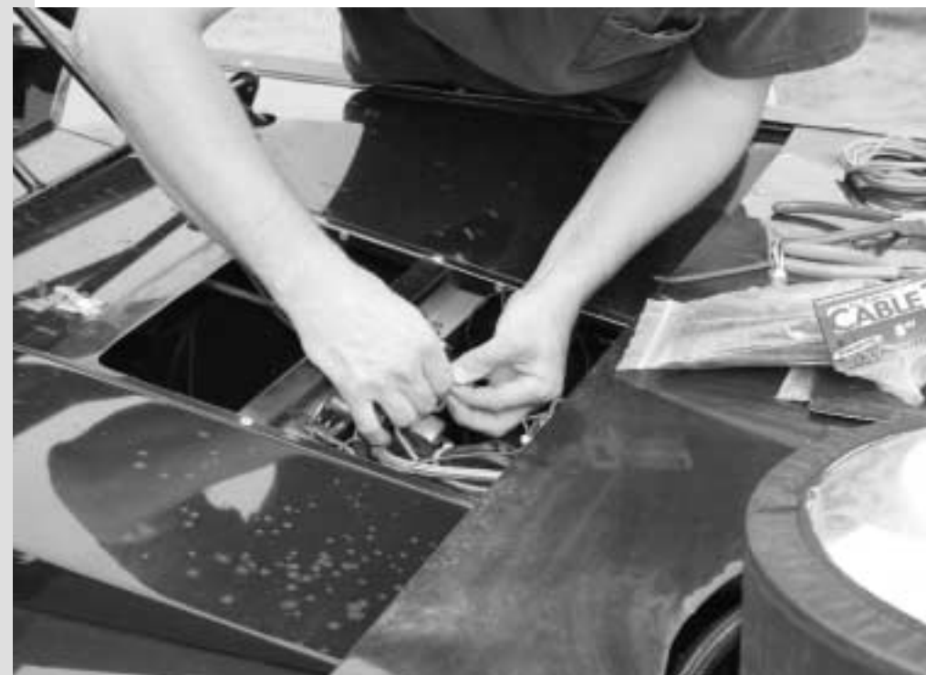
For our test, the traction control unit was installed behind the dash of the car, near the MSD box. With the smaller units, possible mounting points are limitless.
